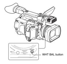
During adjustment, an in-progress message is displayed on the screen. When the adjustment is completed successfully, the message changes to a completion message, and the obtained color temperature is displayed.
